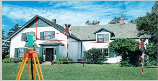
Remote Elevation Measurement
