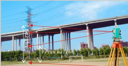
Remote Elevation Measurement
