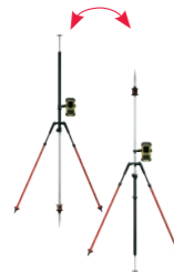
CRP pole Flip pole to get best prism position
