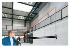
Indirect height measurements using Pythagoras functions.
